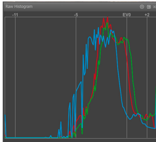
Figure 34. Shot 4018, Raw histogram, blue channel is lagging behind red and green channels
