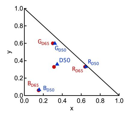
The figure above just plots the xy chromaticities of the primaries under D65 and D50 adaptations. We can see that the adaptation from D65 to D50 is not dramatic but noticeable. An interesting observation is that, in changing the illuminant from D65 to D50, the primaries move roughly along the same direction from D65 to D50.
